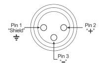
Fig 1. XLR Output Connector Assignment
