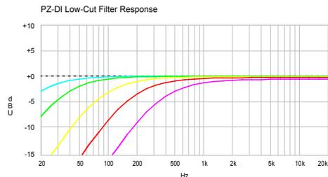
Start by setting the filter control completely counter-clockwise. Slowly turn it clock-wise until you notice the bass roll off. Turn back a bit and you are set. The filter position is usually set in proportion to the size of the instrument whereby larger instruments such as a contrabass will be set with more bass, while a cello or violin will have less.
