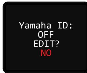
The RMP-D8 will prompt the user to EDIT the Yamaha ID. The default Yamaha ID is set to "OFF" and the EDIT prompt defaults to "NO." To EDIT the Yamaha ID number, rotate the ADJUST wheel one detent clock-wise until the EDIT prompt says "YES." Press the CONFIG button to accept the change.
